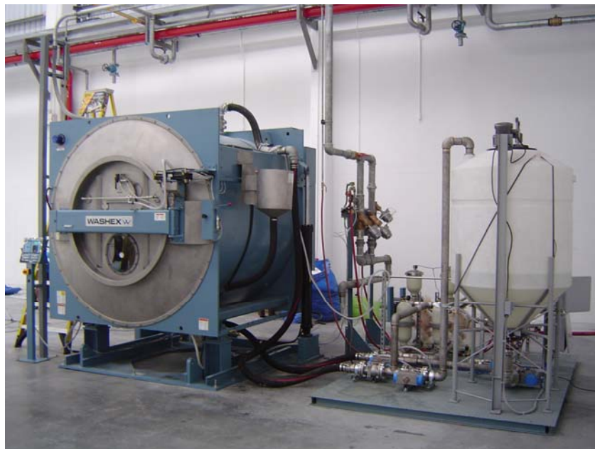
Figure 6. LLIN Chemical Feed System engineered, built and integrated into Washex DPM 5000 washer/extractor by Texchine, Inc.
